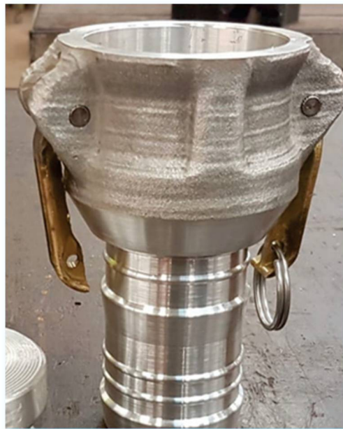
Spee3D Cold Spray copper printed and finished part and Cold Spray Aluminum 6061 Hydraulic Camlock
